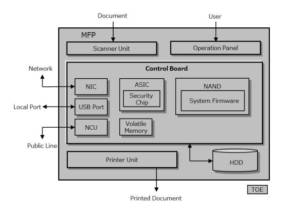
The Operation Panel is the hardware that displays status and results upon receipt of input by the TOE user. The Scanner and Printer units are the hardware that input documents into the TOE and output documents as printed material.
